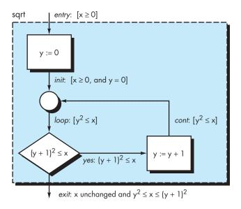
To verify the correctness of this design, entry and exit conditions are added as shown in Figure 28.6. The entry condition notes that x must be greater than or equal to 0. The exit condition requires that x remain unchanged and that y satisfy the expression noted in the figure. To prove the design to be correct, it is necessary to prove the conditions *init*, *loop*, *cont*, *yes*, and *exit* shown in Figure 28.6 are true in all cases. These are sometimes called *subproofs*.
