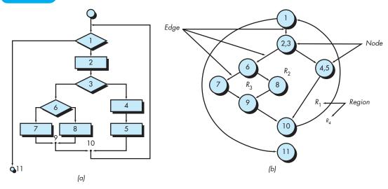
introduced.<sup>3</sup> The flow graph depicts logical control flow using the notation illustrated in Figure 23.1. Each structured construct (Chapter 14) has a corresponding flow graph symbol.
