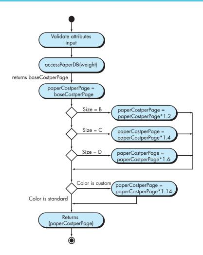
Step 5. Develop and elaborate behavioral representations for a class or component. UML state diagrams were used as part of the requirements model to represent the externally observable behavior of the system and the more localized behavior of individual analysis classes. During component-level design, it is sometimes necessary to model the behavior of a design class.
