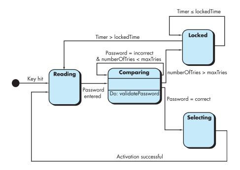
specifying the event that causes the transition to occur, you can specify a guard and an action ICha931. A *guard* is a Boolean condition that must be satisfied in order for the transition to occur. For example, the guard for the transition from the "reading" state to the "comparing" state in Figure 11.1 can be determined by examining the use case:
